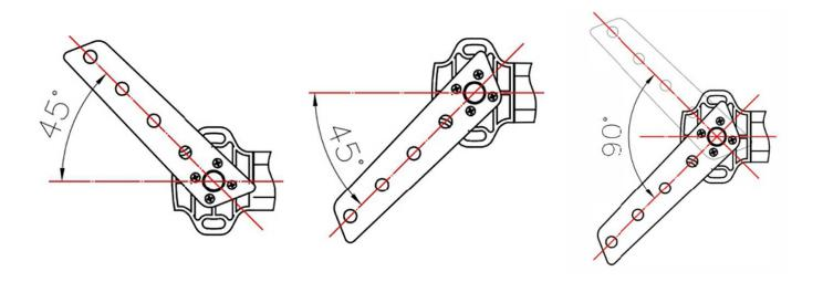
For proper operation, the angle should not exceed 45 degrees from the center on the up or down swing of the arm. You must adjust the height of the suspension within these angle limits by adjusting the attached connecting arm's length or repositioning the mounting arm to the vehicle so that the range of motion from all the way up and all the way down stays within the 90 degree sweep.
